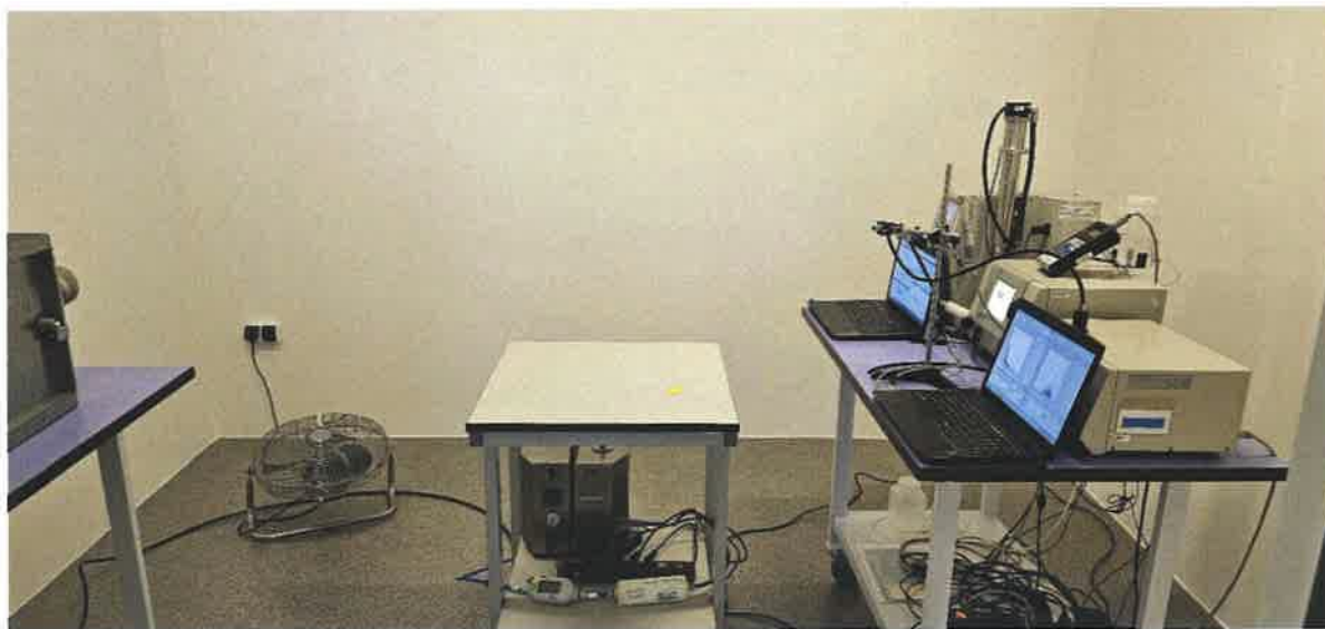
Figure 2.1. View of the test stand for testing nanoparticle emissions from lamp samples
